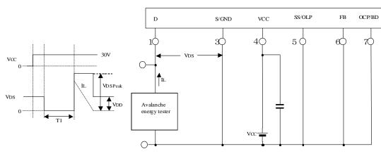
Equation for calculation of avalanche engery,  $E_{AS}$ ; to be adjusted for  $I_L Peak = 5.8 A$
