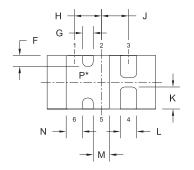
BOTTOM VIEW \*Exposed pad P connects pins 1, 2, 5, and 6.
