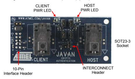
AT88CK109BK3 has two SOT23-3 sockets that support the AT88SA100, AT88SA102, and the AT88SA10HS 3-leads devices.
