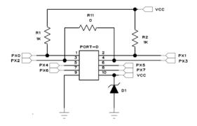
On the AT88CK109BK3, Px2 and Px3 are tied together with a zero ohm resistor (R11). When mounted to the AT88Microbase, pins Px2 and Px3 align with pins (PB3/PD2) and (PB7/PD3). The USART pins, PD2 (RXD) and PD3 (TXD), are effectively tied together with R11allowing the USART to be compatible with the CryptoAuthentication 1-wire interface.
