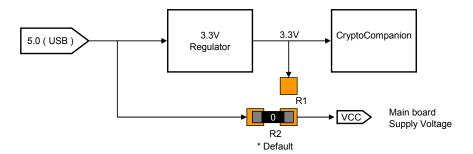
The CryptoCompanion supply voltage is always 3.3V, regardless of R1and R2 configuration.
