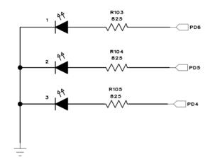
Note: AVR can source or sink enough current to drive an LED directly.
