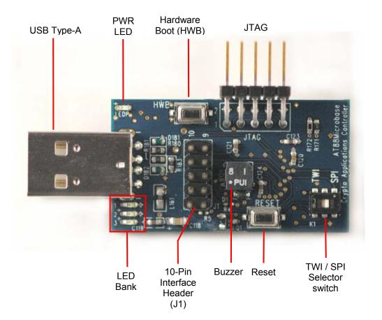
Figure 3. AT88Microbase Components (back side)
