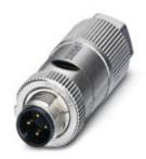
Bus system connector, PROFIBUS PA (31.25 kbps), 2-position, halogen-free, shielded, Plug straight M12, A-coded, Insulation displacement connection, Knurl material: Zinc die-cast, nickel-plated, External cable diameter 5 mm ... 9.7 mm
