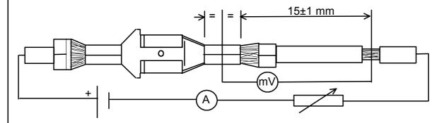
The maximum acceptable values are indicated in the following table (current intensity: A, voltage drop: mV):
