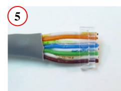
Insert Wires into -A192 Management Bar, maintaining alignment
