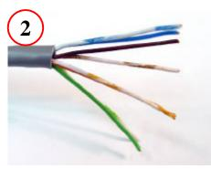
Untwist the pairs and Straighten the Wires
