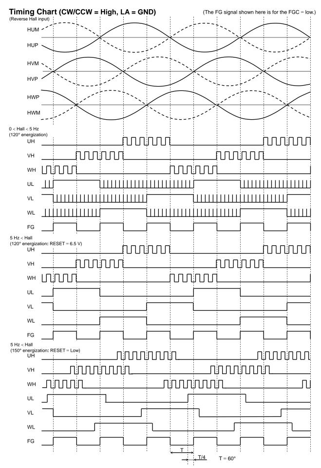
\*: When the Hall signal is 5 Hz or higher, the lead angle function operates in accordance with the LA pin signal. 15
