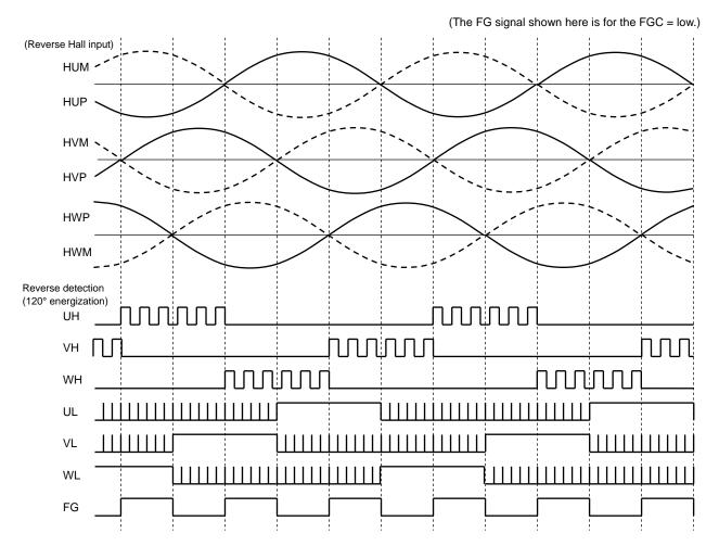
\*: When CW/CCW = Low and a reverse Hall signal is input, the motor runs at 120° energization for a lead angle of 0° (reverse rotation)
