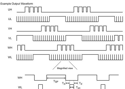
$T_{SP}$ : Variable depending on the  $V_{SP}$  (the figure above being applicable when  $V_{SP} = 5.4 \text{ V (typ.)}$ );  $T_{OD} = 18/f_{OSC}$ ;  $T_{OSC}$ ;  $T_{OSC}$   $T_{OSC}$ ;  $T_{OSC}$
