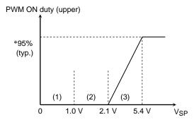
\*: The maximum ON duty is  $T_{ON} = 95\%$  (typ.) when  $V_{SP} = 5.4 \text{ V}$  (typ.). Example: If  $f_{OSC} = 5 \text{ MHz}$ , then ON time = 48  $\mu s$  (typ.) ( $f_{C} = 19.8 \text{ kHz}$ ). If  $f_{OSC} = 4 \text{ MHz}$ , then ON time = 60  $\mu s$  (typ.) ( $f_{C} = 15.9 \text{ kHz}$ )
