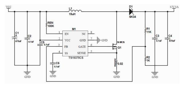
$V_{OUT}$ = $V_{FB}$  x (1+R1/R2),  $V_{FB}$ =1V, R2=1k~3k C4 Capacitor ESR suggest 30m $\Omega$  ~ 100m $\Omega$
