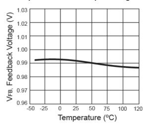
Feedback Voltage vs. Temperature
