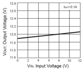
Input Voltage vs. Output Voltage
