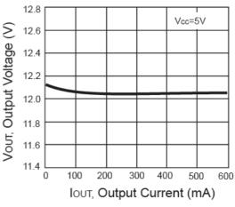
**Output Current vs. Output Voltage**
