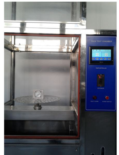
Testing under water jet
