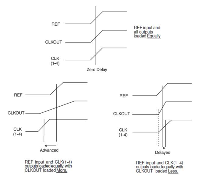
Timing diagrams with different loading configurations
