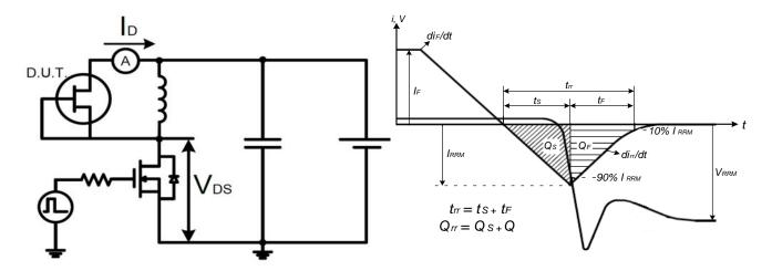
Figure 13. Test Circuit for Reverse Diode Characteristics
