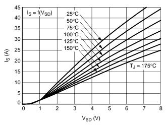
Figure 7. Forward Characteristics of Rev. Diode
