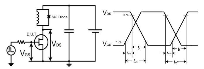
Figure 11. Switching Time Test Circuit
